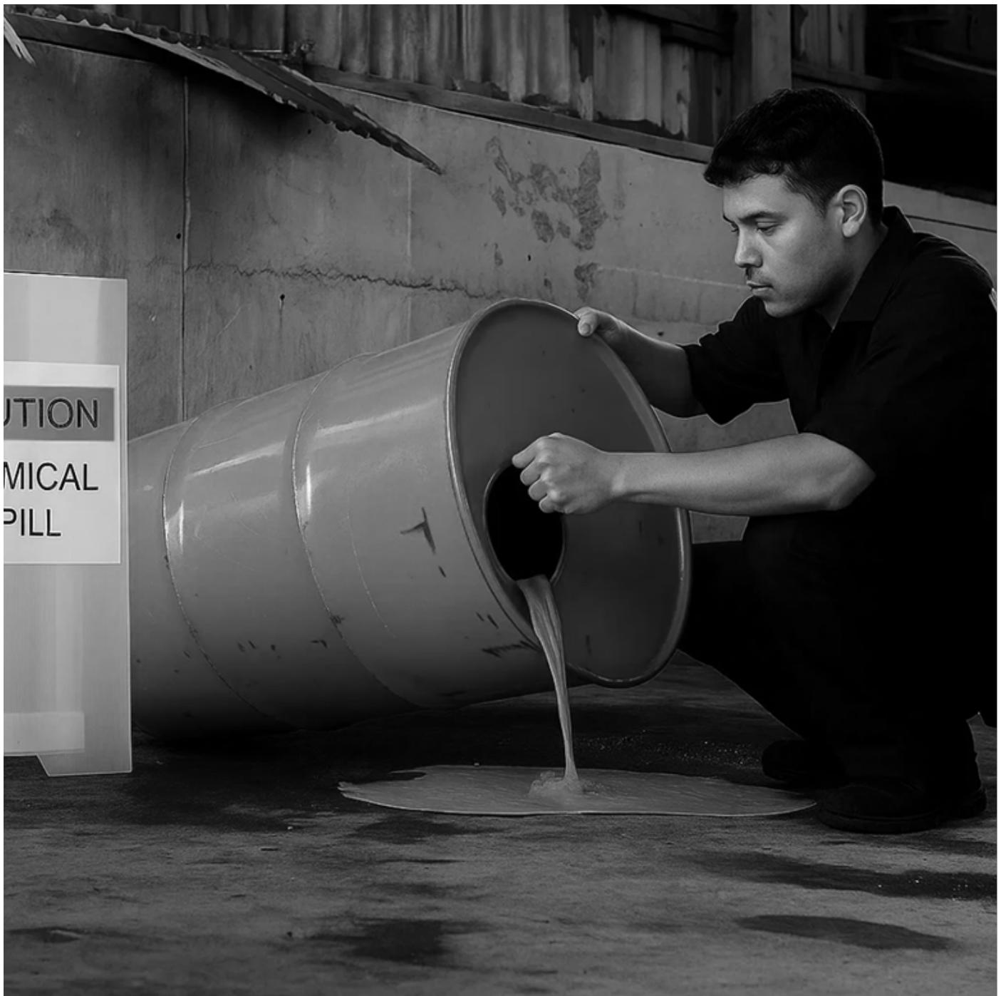
The worker is handling a leaking barrel of hazardous material without wearing any visible personal protective equipment (PPE), such as gloves, eye protection, or protective footwear. The spill is being allowed to spread across the floor, creating a serious slip, chemical exposure, and environmental hazard.
