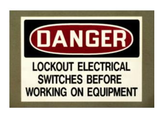
Failure to lock out and tag machinery before working on it is a major cause of injury and death in the United States. Workers can be electrocuted or lose fingers, hands, arms, or suffer severe crushing injuries because machinery is inadvertently turned on while being serviced or maintained. Lockout/Tagout prevents these in juries. This short program is designed to explain basic lockout/tagout procedures, some terminology used in the procedures and general requirements.
