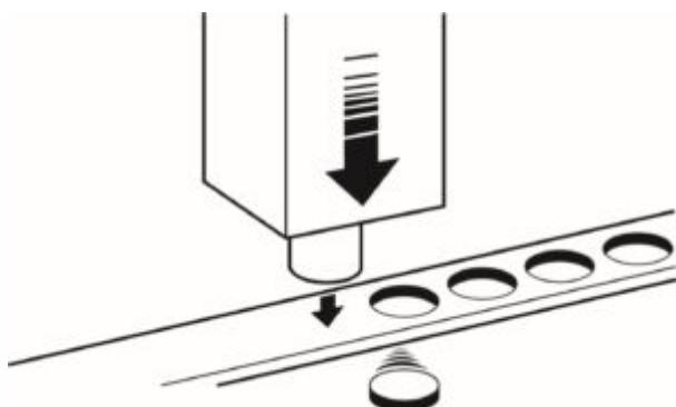
Shearing action involves applying power to a shear or knife to trim or shear materials such as metal. The danger is where stock is inserted, held and withdrawn, as with hydraulically or pneumatically powered shears.
