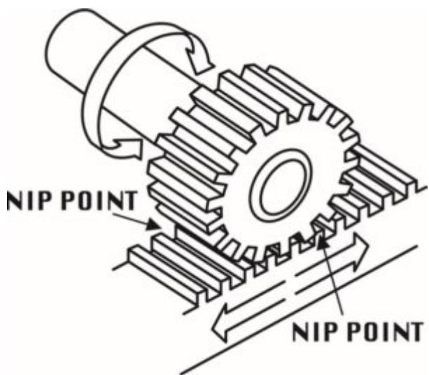
Nip points also occur between rotating and fixed parts, spoked hand wheels on flywheels, screw conveyors and the periphery of an abrasive wheel – and create shearing, crushing or abrading actions.
