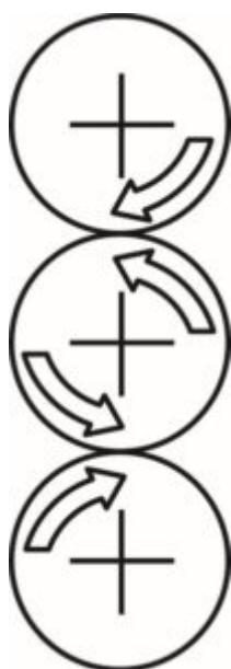
Rotating and tangentially moving parts also cause nip points. Potential hazards include the points of contact between a power transmission belt and its pulley, a chain and its sprocket, or a rack and pinion.
