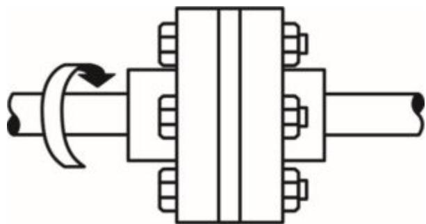
Rotating parts cause hazards such as in-running nip points. There are three main types of in-running nip points. Parts can rotate closely to each other in opposite directions while their axes are parallel to each other. When they run closely, the stock fed between two rolls produces a nip point. This danger is common on machines with intermeshing gears, rolling mills and calendars.
