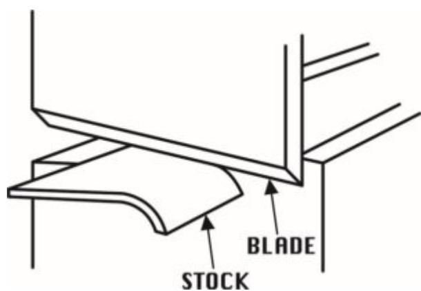
Bending action results when power is applied to a slide to draw or stamp metal or other material. This is a threat where stock is inserted, held and withdrawn, as with equipment such as power presses.
