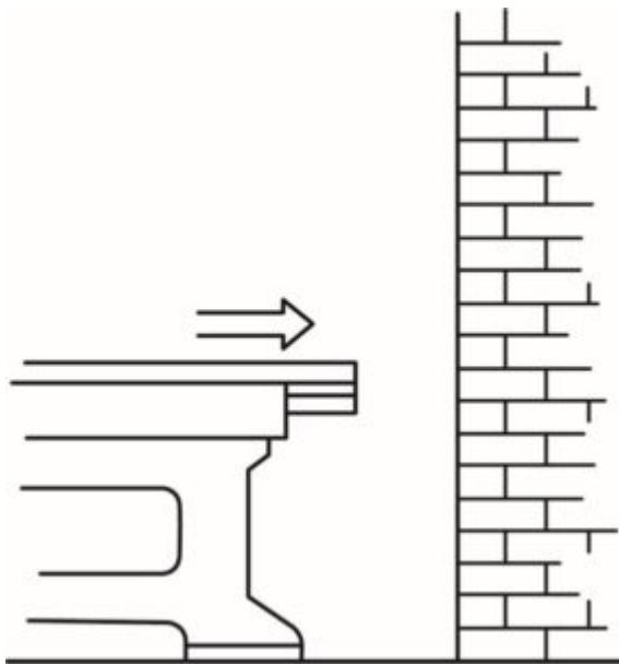
With transverse motion – movement in a straight continuous line – moving parts can catch or strike a worker in a pinch point or shear point.
