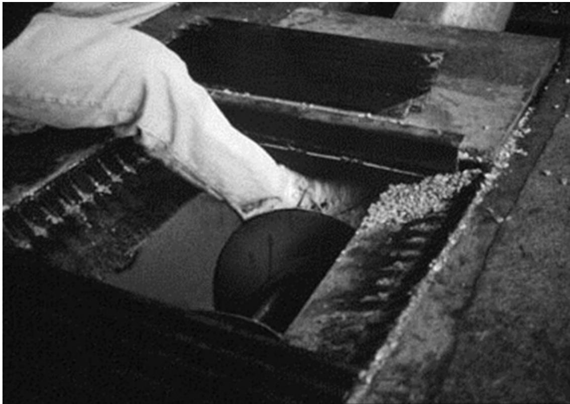
**What's wrong in this picture?** An auger's sharp corkscrew blade rotates as it draws grain up. Coming into contact with an unguarded blade can result in significant lacerations and broken bones which is happening in the picture above.
