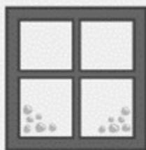
Prevent condensation by reducing humidity, increasing ventilation, or raising the indoor air temperature.
