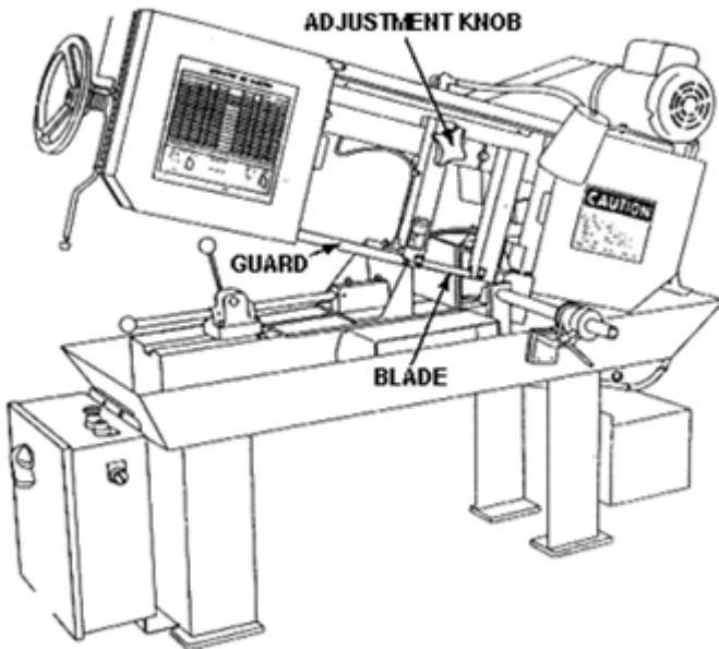
3. Interlocked guards that automatically shut off or stop the machine when a tripping mechanism is activated and keeping it stopped until the guard is put back in place
