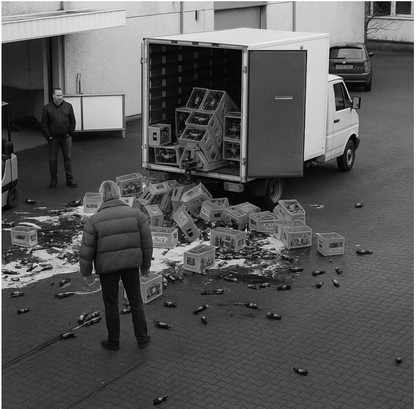
In this image, crates of glass bottles have spilled out of a delivery truck, causing a hazardous mess on the pavement. This incident highlights a major issue in local trucking: improper load storage. Without secure packing, shifting cargo can lead to breakage, financial losses, and serious safety risks to drivers, pedestrians, or nearby workers.
