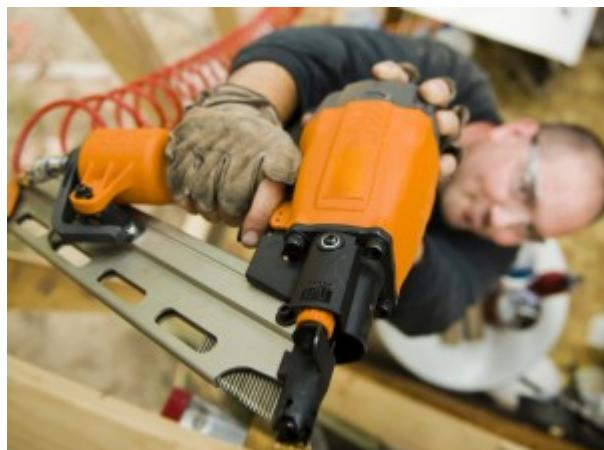
**3. Single Sequence Triggers** which like full sequential triggers, will only fire when the controls are activated in a certain order. First, the safety contact tip must be pushed into the work piece.
