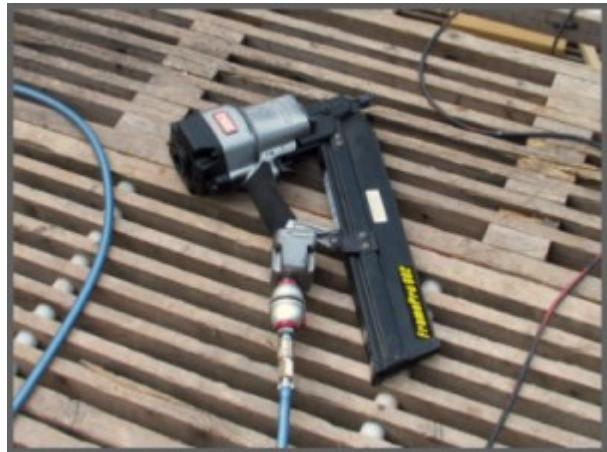
**4. Single Actuation Triggers** which like contact triggers, fire a single nail when the safety contact and trigger are activated in any order but also fire a second nail by releasing the trigger, moving the tool and squeezing the trigger again without releasing the safety contact tip.
