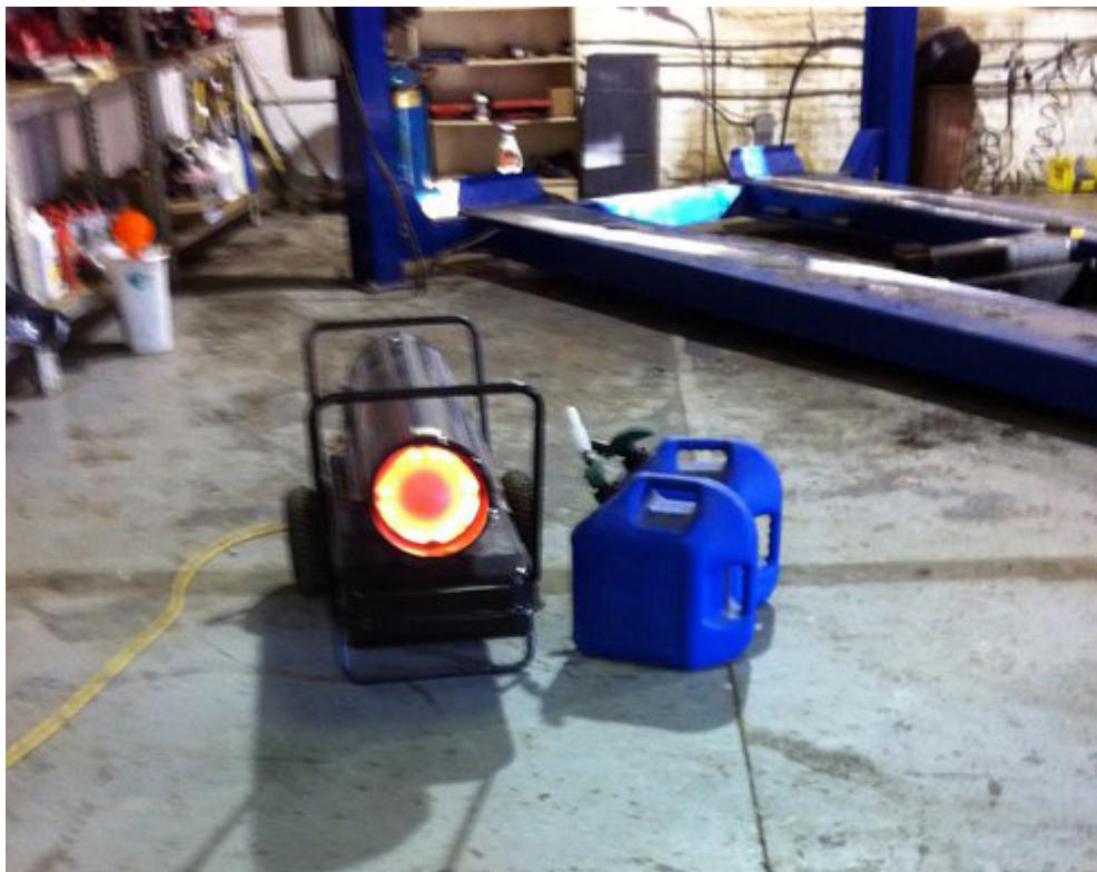
Even a blurry photo can't obscure the danger of placing a kerosene heater inches away from fuel containers. Hopefully, the containers are empty; but even if they are, they may emit flammable vapors that heat from the device could cause to ignite. The electrical cord stretching across the floor as a trip wire/additional source of ignition adds insult to injury.
