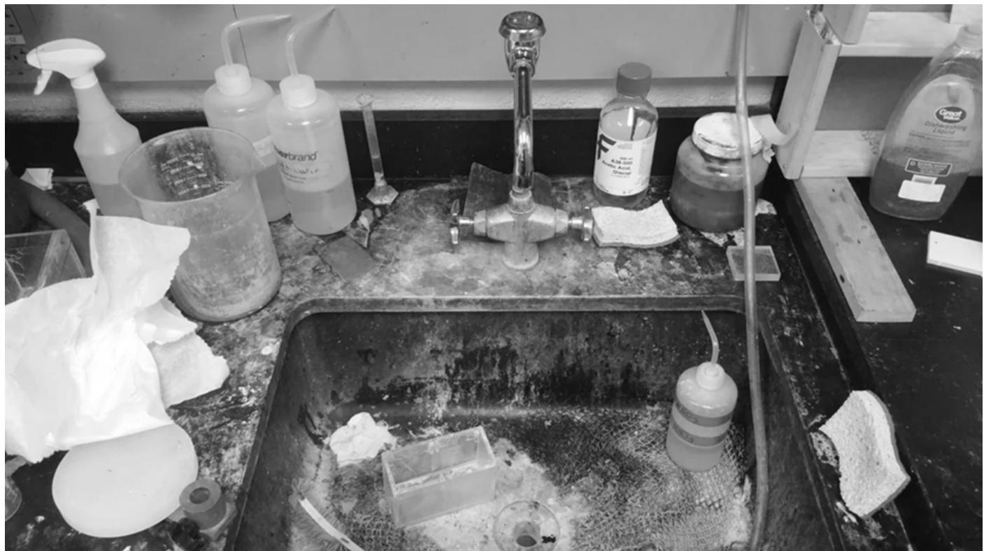
This image shows a major lapse in housekeeping and hygiene in a chemical work area. Contaminated surfaces, unlabelled bottles, and residue buildup around the sink create serious safety risks. Chemicals left unsecured or spilled can lead to cross-contamination, reactions, skin burns, inhalation hazards, and even accidental poisoning. Poor hygiene in such areas also increases the likelihood of environmental contamination and regulatory violations.
