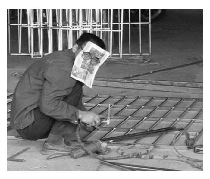
What is wrong in this picture? There is a guy working on welding with any proper PPE. He is using a paper to protect his face from carbon monoxide exposure.
